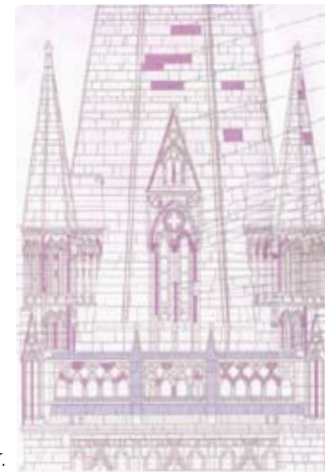
The Photogrammetric Survey has helped identify the damaged stones that need replacing on the central tower.
